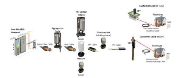
The following diagram sets out the CP network/backhaul at a specific Openreach 'Point of Handover' (Exchange):
